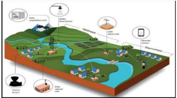
Figure 4: Working principle of the established CBFEWS instrumentation & layout.
