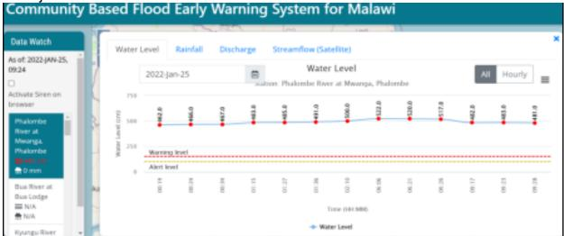
Figure 2: Status Water level in Phalombe river passed the warning level for the warning that was issued 24 hours ago (24<sup>th</sup> January at 08:00am).
