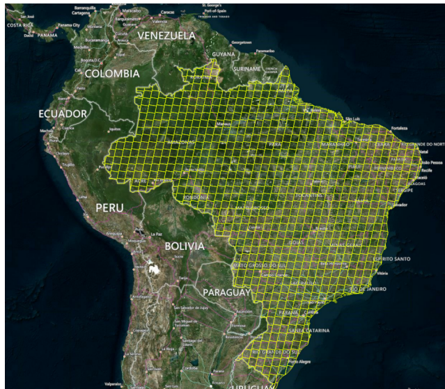
Figure 2: CBERS-4 WRS Grid for MUX
