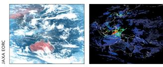
Himawari-8 geostationary satellite delivers aerosol data every 10 minutes with 5km resolution. Hot spot detection and forest fire monitoring are conducted using other low Earth orbiting satellites, together contributing to estimates of particulate matter.
